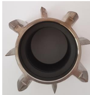
Extruder with Carbon Bearing Pressed Into Place
